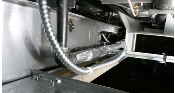
Figure 3: The return manifold is easily accessible on the right side of the fryer.
